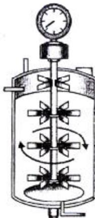
Ans. Simple stirred tank bioreactor = 1
